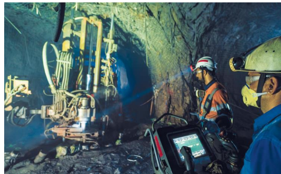
Long-haul drilling machine at work
