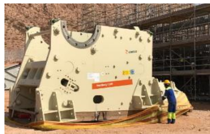
Jaw Crusher Delivered to Site
