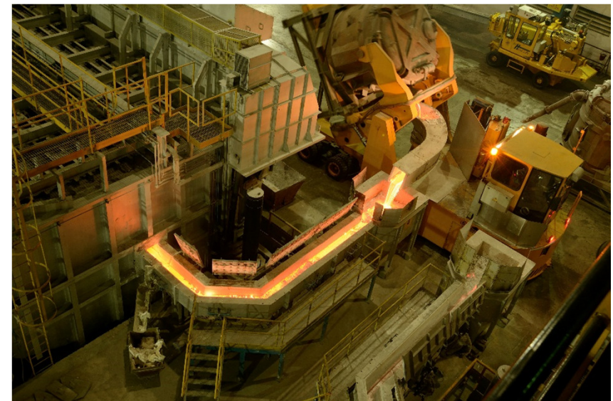
Molten Aluminium being poured in a Casting Machine at Jharsuguda
