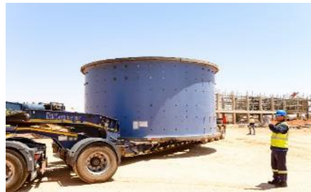
Mill shell on site
