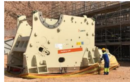
Jaw Crusher Delivered to Site
