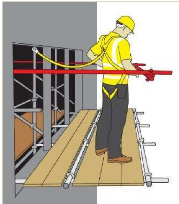
(iii) Needles are boarded out to create a scaffolders' safe zone to complete the truss-out scaffold.
