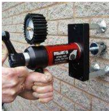
Figure29: AnAnchorTesting Devicehelpsinensuring whethertheinstalledanchors areadequateornot
