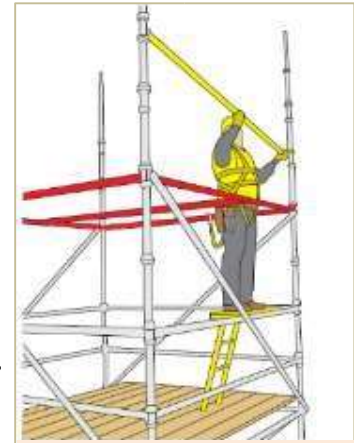
Figure 66: Scaffolder installing a guardrail in advance to the next lift from a scaffolders' step protected by the ledgers and transoms
