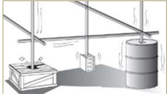
Figure 11: Unsuitable bases supports
