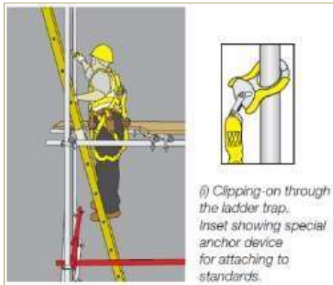
Figure 76: Special snap-hooks for anchoring onto the vertical scaffold tubes
