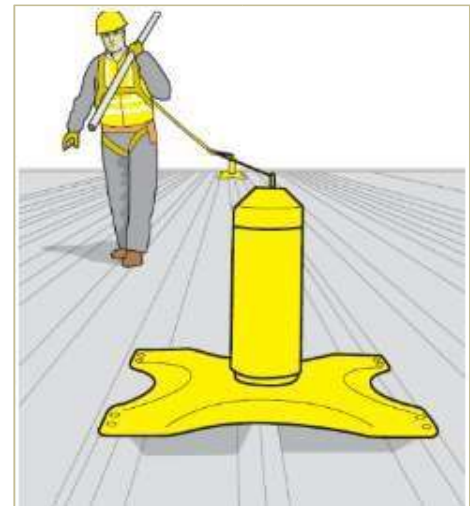
Figure 96: Scaffolder utilizing an installed protection system for roof
