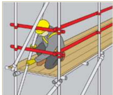
Figure 40: Safe handling bay (with double guardrails, stop ends returns) - used for raising and lowering materials.
